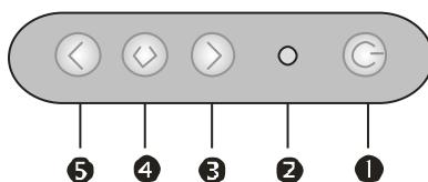
**①POWER SWITCH:** Pushing the power switch will turn the monitor on.
