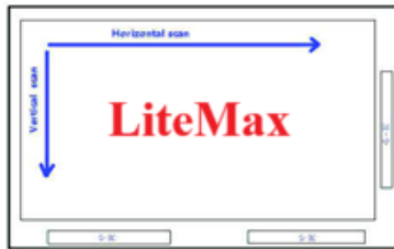
Fig. 1 Normal scan (Pin24, Reverse = Low or NC)
