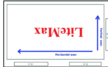
Fig. 2 Reverse scan (Pin24, Reverse = High)
