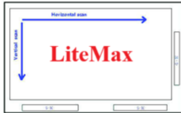
Fig. 1 Normal scan (Pin24, Reverse = Low or NC)
